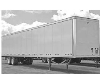
(10) '20 Vanguard VXP, 53'x102", air ride, sldg. tdm., swg. doors, alum. roof. Due in March.
