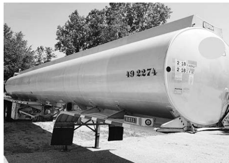
'93 Heil, 9400-gal., tdm., 1-compt., btm. load, alum. composition, fixed axle, air ride susp., vapor recovery, alum. whls., call.
