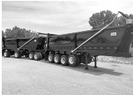
'21 E-PAK super train, HARDOX 1/4 AR450, 28' lead, 26' pup, steel disc whls., Reyco 21B & Meritor lifts, remote grease blocks, tarps installed, ON ORDER.
