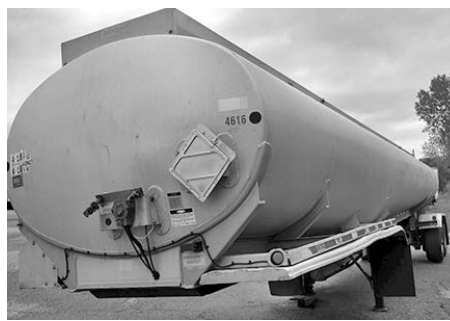
'98 Frue., 9400x4-compt., tdm. on spgs., water trlr.
