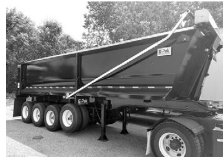
'21 E-PAK, 28' lead, air assist gate, HARDOX 1/4" AR450, 4-axle, (1) lift, steel disc, remote grease, Aero tarp, ON ORDER.
