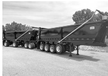
'19 E-PAK super train , HARDOX 1/4 AR450, 28' lead, 26' pup, steel disc whls., Reyco 21B & Meritor lifts, remote grease blocks, tarps installed, IN STOCK.
