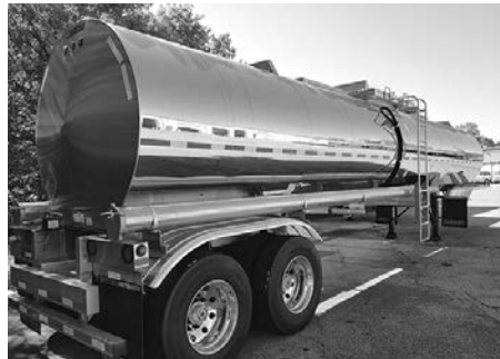
'20 Brenner, 7000-gal., D.O.T. 407, air ride, rear discharge, in-transit heat, alum. whls.
