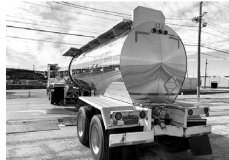
'84 STE, 5300-gal., S.S., rear discharge, on spgs.
