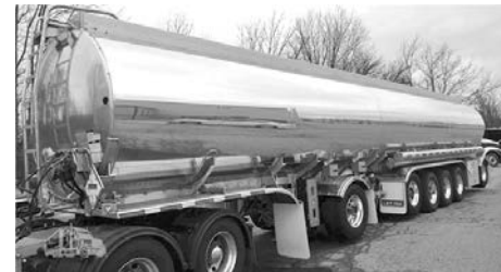
'21 LBT 9-quad-9, 5-compt., 6-axle, air ride, disc brakes, alum. whls., hose trays, vapor recovery.
