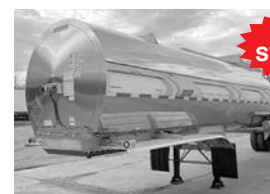
'24 Brenner 7000-gal. DOT 407 316SS, rear discharge, intransit heat, 13 lb. product wt./U.S. gal., (2) clean outs, Betts hyd. pump & hydrolet valve, Girard pressure release vent, HEND. Intraax air ride susp., alum. whls. $87,500 incl. F.E.T.
