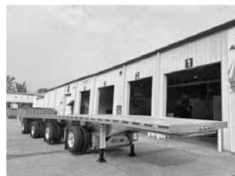
'24 Extreme 50' x102" quad axle trlr., 14" coil well, air ride susp., (2) lift axles, alum. whls., call for price.
