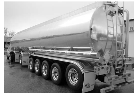
'21 LBT, SIX ON ORDER, 13,400-gal., 5-compt., all air, (3) lifts, S.S. frame, disc brakes, pol. barrel, alum. whls., MANY EXTRAS, call for details.
