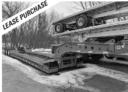
'19 Fontaine 55L Plus, 55-ton, tri-axle, 3rd axle lift, 26' well, 18" deck ht., O/S alum. whls., (14) pr. lash rings, 2" floor, (2) position king pin, call for details.
