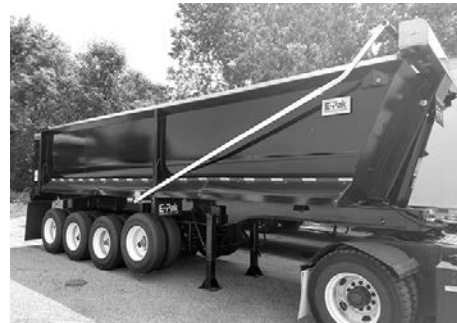
'19 E-PAK , 28' lead, air assist gate, HARDOX 1/4" AR450, 4-axle, (1) lift, steel disc, remote grease, Aero tarp, IN STOCK.
