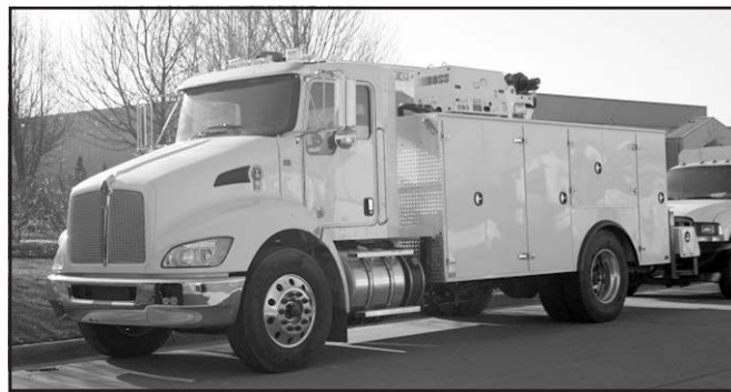
'18 KW T370, 12.5F, 21R, Paccar PX-9, Meritor MFS12E frt. axle, 5.57 ratio, Meritor MS21-14x4 rear axle, 6 spd., Allison 3000RDS, 188" WB, stk. #K6637.
