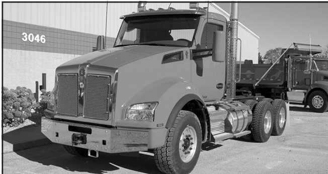
'18 KWT880, X15 1850 lb. ft. Cum., 565 hp, dsl., tdm., 18 spd. O.D., eng. brake, 3.91 ratio, 385/65R22.5-18 Michelin XZY3 frt., 11R22.5-16 Michelin XDEMS tires, 192" WB, 64,000 GVW, 20F, #K50950.
