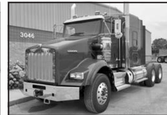
'18 KW T800, 14.6F, 46R, Cum. X15, Dana Spicer E-1462W frt. axle, 3.73 ratio, Meritor RT46-160P rear axle, 62" slpr., Fuller RTLO18918B, 224" WB, stk. #K51060.
