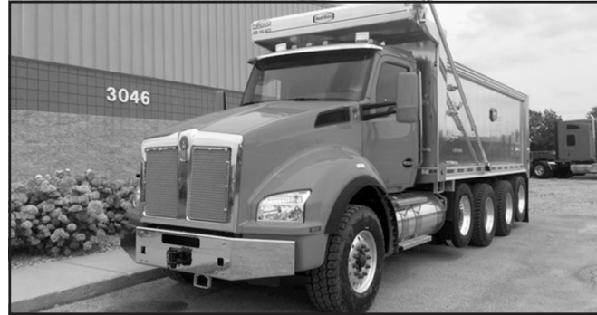
'18 KW T880 , 19'6" length, Cum. X15, 565 hp, dsl., quad axle, viper red color, 18 spd. O.D., eng. brake, 3.91 ratio, 385/65R22.5-18 frt. tires, 11R22.5-16 rear tires, 205" WB, 64,740 GVW, 20F, stk. #K50980.
