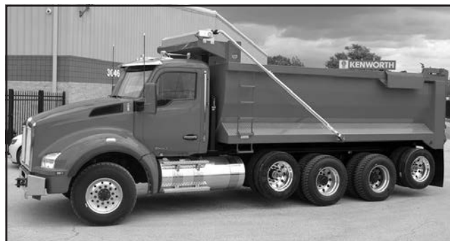
'18 KWT880, viper red, 20F, 46R, Cum. ISX15, Dana Spicer D2000 frt. axle, 4.10 ratio, Dana Spicer D46-170HP rear axle, 18 spd., Fuller RTLO-18918B, stk. #K50952.
