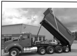
'18 KW T880, 20F, 46R, Cum. ISX15, Dana Spicer D2000 frt. axle, 4.10 ratio, Dana Spicer D46-170HP rear axle, 18 spd., Fuller RTLO18918B, 205" WB, stk. #K50980.
