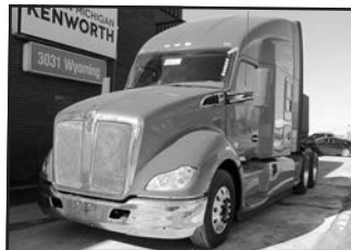
'18 KW T680 , 53,200 GVW, 100 miles, 13.2F, 40R, Cum. IX 15, Meritor MFS13 frt. axle, 3.36 ratio, Meritor MT40-14X3 rear axle, 76" slpr., 13 spd. Fuller RTLO18913A, stk. #K51028.
