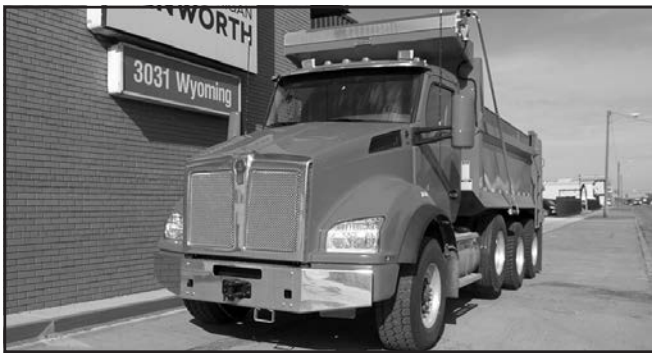
'18 KW T880, 20F, 46R, Paccar MX-13, Meritor MFS20 frt. axle, 3.91 ratio, Meritor RT46-160P rear axle, Ultrashift, Eaton FO16E313A-MHP trans., 200" WB, stk. #K51079.
