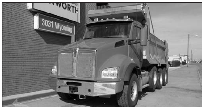
'18 KW T880, 20F, 46R, Paccar MX-13, Meritor MFS20 frt. axle, 3.91 ratio, Meritor RT46-160P rear axle, Ultrashift, Eaton FO16E313A-MHP trans., 200" WB, stk. #K51079.
