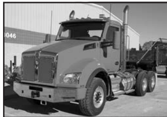
'18 KW T880, 100 miles, 20F, 46R, Cum. ISX15, Dana Spicer D2000 frt. axle, 3.91 ratio, Dana Spicer D46-170HP rear axle, 18 spd., Fuller RTLO18918B, stk. #K50950.
