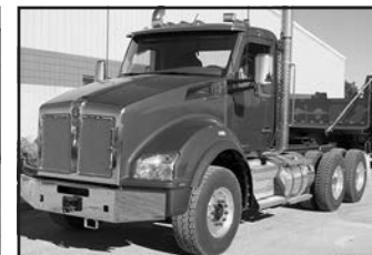
'17 KW T880, ISX-15 1850 lb. ft. Cum., 560 hp, dsl., tdm., 18 spd. O.D., eng. brake, 3.91 ratio, 385/22.5-18 steer, 11R22.5 rear tires, 191" WB, 66,000 GVW, 20F, 46R, #K50930.
