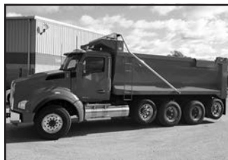
'18 KW T880, 19' length, ISX15 1850 lb. ft. Cum., 560 hp, dsl., 18 spd. O.D., eng. brake, 4.10 ratio, 385/65R22.5-18 Michelin XZY3 frt., 11R22.5-16 Michelin XDEMS rear, 205" WB, stk. #K50952.
