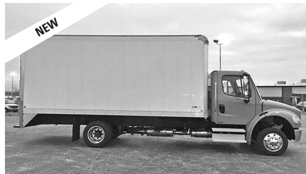
New FTL M2-106 , Cum. ISB, Allison auto, under CDL, 18' van body w/rear step bumper.
