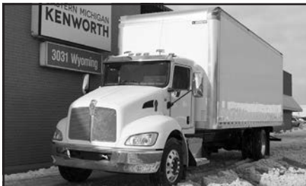
'17 KW T270, Paccar PX-7, Dana Spicer E-10021 frt. axle, 5.57 ratio, Dana Spicer IP22060S rear axle, 5 spd., Allison 2500RDS, 272" WB, stk. #K6517.
