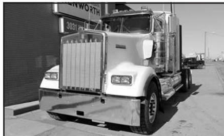
'18 KW W900, 100 miles, 14.6F, 46R, Cum. ISX15, 18 spd., Dana Spicer E14521 frt. axle, Dana Spicer D46-170HP rear axle, Fuller RTLO18918B, 240" WB, stk. #K50954.
