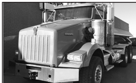
'14 KW T800B, Ultrashift, Cum. ISX15 dsl., 600 hp, tdm., eng. brake, 3.91 ratio, 385/65R22.5 frt. tires, 11R22.5 rear tires, 191" WB, 62,000 GVW, 20F, 46R, stk. #P0415.
