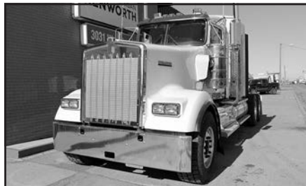
'18 KW W900, 100 miles, 14.6F, 46R, Cum. ISX15, 18 spd., Dana Spicer E1452I frt. axle, Dana Spicer D46-170HP rear axle, Fuller RTLO18918B, 240" WB, stk. #K50954.
