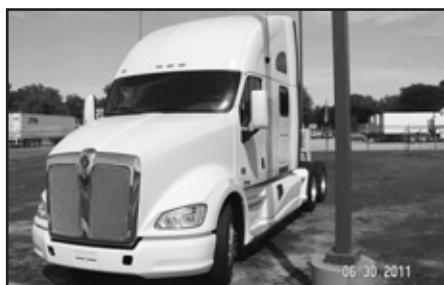
New '12 KWT700 , 75" raised roof condo, ISX Cum., 525 hp, dsl., 18 spd. O.D., eng. brake, air ride susp., 22.5 LP tires, alum. whls., 234" WB, tdm., 13.2F, 40R.
