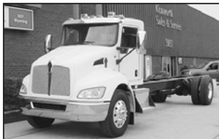
New '12 KW T270 , PX6 Paccar, 240 hp, dsl., auto., air ride susp., 5.57 ratio, 11R22.5 tires, alum. O/S whls., 272" WB, S/A, 16R, 10F.
