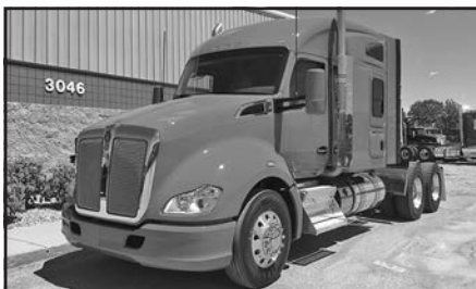
'18 KW T680, 13.2F, 40R, Cum. X15, frt. axle Meritor MFS13, rear axle Meritor MT40-14X3, Fuller 13 spd., RTLO18913A, stk. #K51027.
