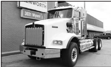
'18 KW T800, Cum. X15, 565 hp, dsl., tdm., 18 spd. O.D., eng. brake, 3.91 ratio, 385/65R22.5 Goodyear frt. tires, 11R22.5 Michelin rear tires, 195" WB, stk. #K51087.
