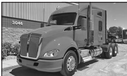
'18 KW T680, 13.2F, 40R, Cum. X15, frt. axle Meritor MFS13, rear axle Meritor MT40-14X3, Fuller 13 spd., RTLO18913A, #K51027.
