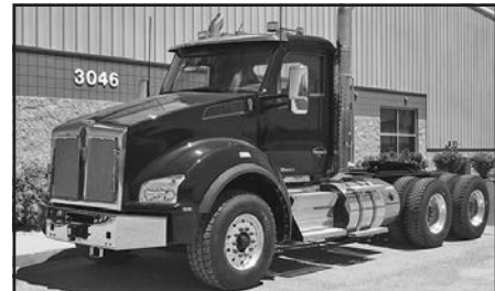
'18 KW T880, Cum. X15, 20F, 46R, 3.91 ratio, frt. axle Dana Spicer D2000, rear axle Meritor RT46-460P, Fuller 18 spd., RTLO18918B, 192" WB, #K50988.
