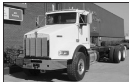
New '12 KW T800 , ISX15 Cum., 450 hp, dsl., 8LL O.D., eng. brake, spg. susp., 3.91 ratio, 22.5 tires, alum./steel whls., 268" WB, tdm., 20F, 46R, great roll-off chassis.
