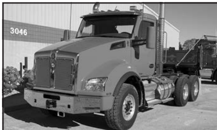
'18 KW T880, 20F, 46R, Cum. ISX15, 3.91 ratio, frt. axle Dana Spicer D2000, rear axle Dana Spicer D46-170HP, Fuller 18 spd., RTLO18918B, #K50949.
