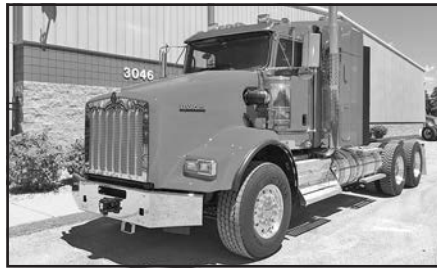
'18 KW T800, Cum. X15, 14.6F, 46R, 385/65R22.5 Goodyear frt. tires, 11R22.5 Goodyear rear tires, 3.91 ratio, Fuller 18 spd., stk. #K51018.
