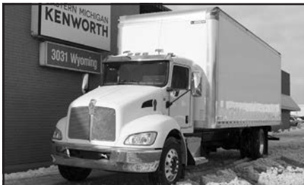
'17 KW T270, Paccar PX-7, Dana Spicer E-1002I frt. axle, 5.57 ratio, Dana Spicer IP22060S rear axle, 5 spd., Allison 2500RDS, 272" WB, stk. #K6517.
