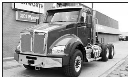
'17 KW T880, ISX 15 1850 lb. ft. Cum., 560 hp, dsl., tdm., 18 spd. O.D., eng. brake, 3.91 ratio, 191" WB, 64,000 GVW, 20F, 46R, #K50899.
