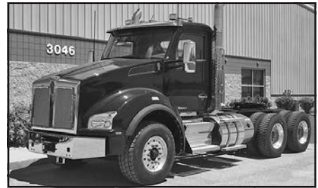
'18 KW T880, Cum. X15, 20F, 46R, 3.91 ratio, frt. axle Dana Spicer D2000, rear axle Meritor RT46-460P, Fuller 18 spd., RTLO18918B, 192" WB, stk. #K50988.
