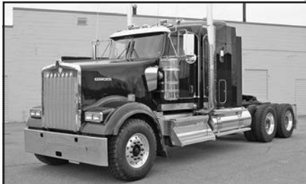
'18 KW W900, 14.6F, 46R, Cum. X15, Dana Spicer E-14621 frt. axle, 3.91 ratio, Dana Spicer D46-170HP rear axle, 18 spd. Fuller, 240" WB, stk. #K51036.
