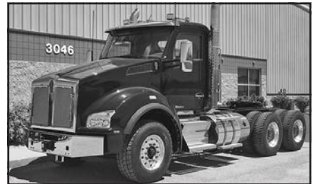
'18 KW T880, Cum. X15, 20F, 46R, 3.91 ratio, frt. axle Dana Spicer D2000, rear axle Meritor RT46-460P, Fuller 18 spd., RTLO18918B, 192" WB, stk. #K50988.
