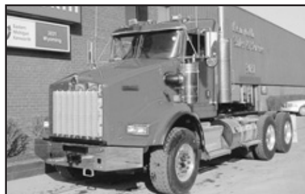
New '12 KW T800 , ISX15 Cum., 550 hp, dsl., 18 spd. O.D., eng. brake, air ride susp., 3.91 ratio, 22.5 tires, alum. O/S whls., 186" WB, tdm., 20F, 46R.
