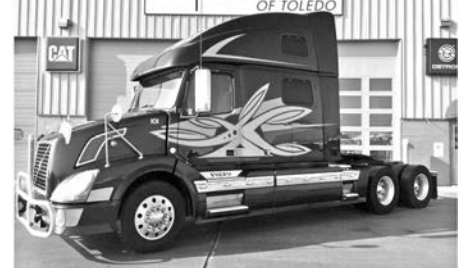
'07 Volvo VNL780, Volvo D16, 535 hp, Eaton 13 spd., Hend. steer axles, Meritor rear axles w/3.42 ratio, 12.5F, 40R, 275/80R22.5 tires, air slide 5th whl., pop-up table in bunk, alum. whls., dual 150-gal. tanks, $19,995.
