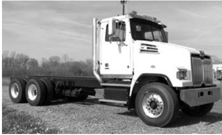
'2016 Western Star 4700SF , DD13 Det., 470 hp, Jake, 8LL trans., air ride, 4.30 ratio, 385 ft. & 11R22.5 rear tires, 152" C.A., 100" A.F., EV4 7 yr./250K ext. eng. warranty, $118,638 + tax.
