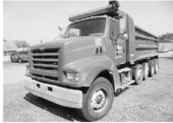
'99 Sterling LT9513 quad-axle, C12 Cat, 435 hp, 8LL trans., 16F, 46R, 18' steel dump bed, 272,000 miles.
