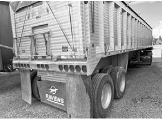
'23 Ravens 36'x102"x60" alum. dump, air ride, elec. tarp, 11R22.5 tires on all alum. whls.
