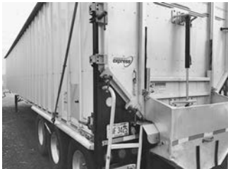
'15 Western Commodities Express 48'x102"x90", air ride, Super Singles on alum. whls., (2) lift axles.
