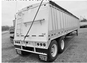
'16 Cornhusker 42'x72" hopper, air ride, 11R22.5 tires on alum. whls. Also: '10 & '01 Cornhusker hoppers.
