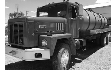
'87 Int'l. Paystar, DT530, 8LL trans., 20F, 44R, 110-barrel vacuum tank.
