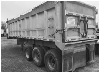
'95 MAC 32'x30" tri-axle dump, alum. frame, air ride, 11R22.5 tires on alum. whls., 2-way gate, lift axle. Also: '00 Benson 22'x66" tdm. alum. dump.
