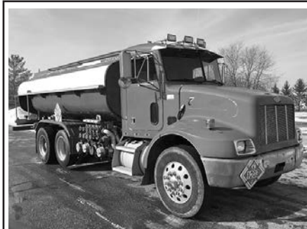
'00 Pete 330, Cat C7, 250 hp, lift axle, 2600-gal., 4-compt., alum. tank, btm. loading, dual delivery system, new hoses & hose reels & nozzles, ready to work, $39,500.
