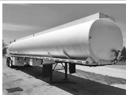
'94 Frue. 9200-gal., 4-compt., clean southern trlrs., DOT306, alum. tank, btm. loading, (5) to choose, starting at $19,900.
