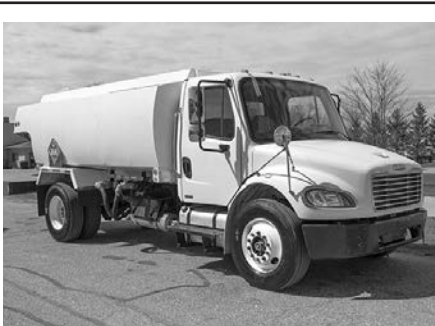
'05 FTL M2 106, Cat C7 dsl., 6 spd., extra clean southern truck, 2800-gal. DOT-306 alum. tank, 4-compt., dual delivery system, 348,000 miles, #SC1332, $49,500.
