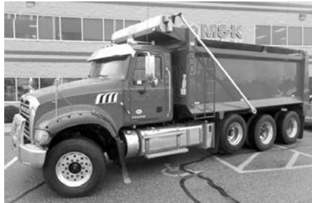
'15 Mack Granite GU713, Mack MP8, 455 hp, dsl., 8LL, tri-axle, 17'6" Bibeau steel body, 18F, 46R, 20K lift axle, 385/22.5 tires, stk. #U9942, $118,950.
