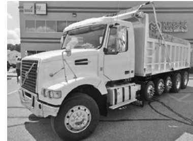
'14 Volvo VHD84F200 5-axle alum. dump, D13, 475 hp, Eaton RTO16908LL trans., T-ride, 20F, Rogers alum. body, 20'5"x95"x51", #U10001, $126,950.
