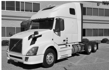
'13 Volvo VNL64T670EX tdm. axle slpr., Volvo D13, 13.0L 6 cyl., 425 hp, 12 spd. I-shift O.D., PS, 221" WB, alum. 22.5 LP tires, 61" dbl. deck condo, 2.64 ratio, 12.35F, 35R, air susp., air brakes, A/C, #U9813, $46,000.
