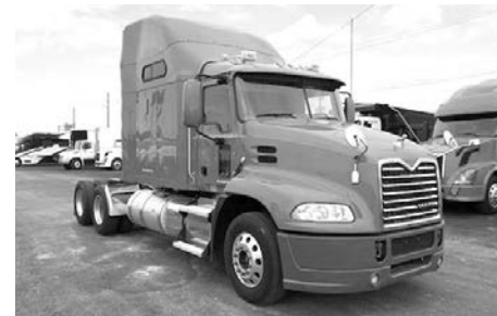
'13 Mack CXU613 tdm. axle slpr., Mack MP8, 445 hp, 6 cyl., dsl., I-shift, 12 spd. O.D., Jake, cruise, PS, Eaton rears, 3.08 ratio, 12F, 40R, alum. whls., air slide 5th whl., 295R22.5 tires, air brakes, A/C, 70" mid-roof slpr., #U9831, $38,950.
