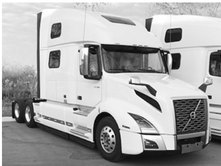
(3) New '18 Volvo VNL860 , D13 500 hp, 2.64 ratio, I-shift, VADA system, disc brakes, bunk heater & inverter.
