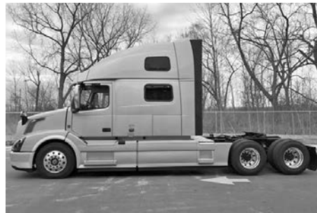
New '18 Volvo VNL64T780 , Volvo D13, 500 hp, I-shift, 239" WB, air ride, 3.08 ratio, stk. #RN1019.
