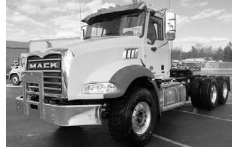
New '16 Mack GU813 , Mack MP8 505 hp, Eaton Fuller 13 spd., Jake, 3.91 ratio, air ride, alum. whls., air slide 5th, 189" WB, stk. #N12446.
