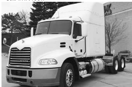
'14 Mack Vision CX613 , Mack MP8, 445 hp, Jake, 10 spd., 3.25 ratio, locking diff., 12F, 40R, alum. whls., 60" slpr., 550,000 miles, #SHU1095.
