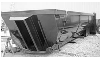
Rugged 24' AR450 steel dump body, 60" sides, air assist high liftgate.
