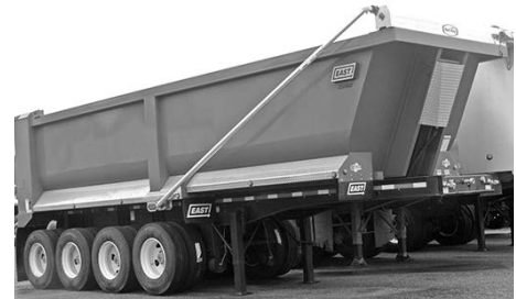
New '18 East AR450 quad axles, high liftgates, 102" wide chassis.
