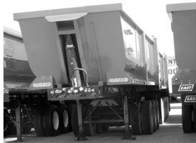
Frue. frame w/new rugged AR450 steel bodies.
