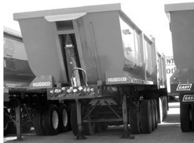
Frue. frame w/new rugged AR450 steel bodies.
