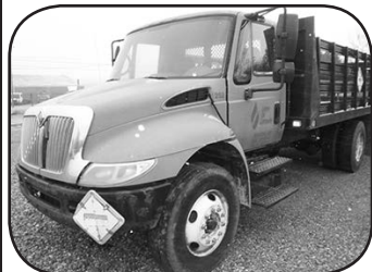
'03 Int'l. 4400 , Int'l. DT466, Fuller 6 spd., 16' stake body w/liftgate, air brakes, 34,000 GVW.
