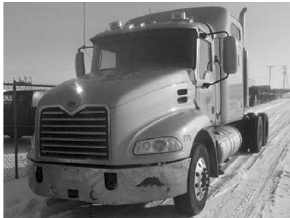
'07 Mack Vision, Mack L6, 12.0L eng. core, RTLO16913A trans., Rockwell 20145 rear, 3:73 ratio, cab & hood.
