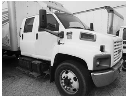
'07 GMC C7500 quad cab, 7.8L Duramax eng. core, Eaton 19060S rear, 5:29 ratio, cab & hood.
