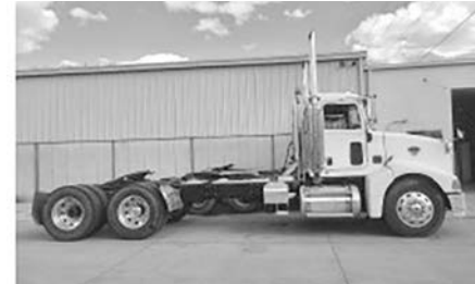
'07 Pete 385 , clean day cab, LWB, 592,000 miles, Cat C13, 430 hp, KCB65723 w/Jake, FRO16210C trans., 12.6F, Eaton DSP40, 3.70 ratio, 162" C.A., 214" C.F.
