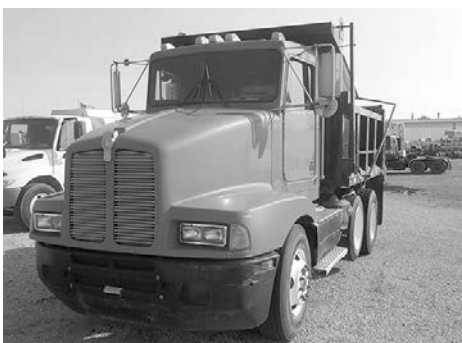
'95 KW T400, L10 260 Cum., Fuller 9 spd., 10' dump, sgl. drive axle w/pusher lift axle.
