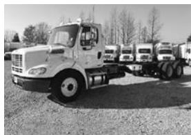
(2) '12 FTL M211264S, DD13, 350 hp, eng. brake, 10 spd., 12F, 40R, air ride cab & susp., 3.90 ratio, 292" WB, 226" C.T., 274,000 & 301,000 miles.
