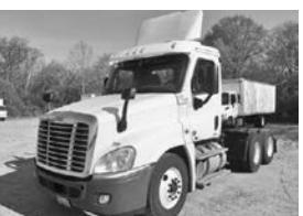
'11 FTL PX12564 ST Cascadia, DD13/450 hp, eng. brake, 10 spd., 12F, 40R, 3.70 ratio, air ride cab & susp., 178" WB, 247,602 miles.
