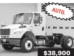
'13 FTL M2 106 S/A tractor, ISC 300 hp, 5 spd. Allison auto., 12F, 23R, air ride cab & susp., 5.22 ratio, 165" WB, 192,507 miles.
