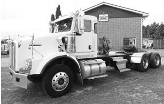
'05 KW T800 day cab, Cat 475 hp, 18 spd., 14.6F, 46R, lockers, 2X frame, $49,500 U.S.
