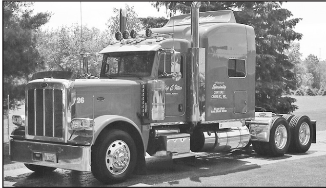
'17 Pete 389 , viper red in color, fully loaded, O/O specs, 78" Unibilt Ultra cab w/platinum int., Cum. ISX 525 hp, 18 spd., 3.55 ratio, air ride, 260" WB, premium steer & drive tires, (10) alum. whls., leather seats & steering whl., keyless entry, Smartnav system, factory aux. heater, fresh D.O.T., 76,000 miles, this is a very clean 1-owner/1-driver truck in exc. cond. w/all service records, super low miles, showroom clean & new truck smell, $149,900.
