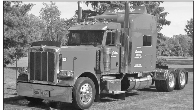
'13 Pete 389 , viper red in color, fully loaded, O/O specs, 70" Unibilt Ultra cab w/platinum int., Cum. ISX 525 hp, 18 spd., 3.55 ratio, air ride, 275" WB, premium steer & drive tires, (10) alum. whls., leather seats, keyless entry, factory aux. heater, new DPF unit, fresh D.O.T., 448,276 miles, this is a very clean 1-owner truck in exc. cond. w/all service records, nice ride w/Smartnav system, $109,900.
