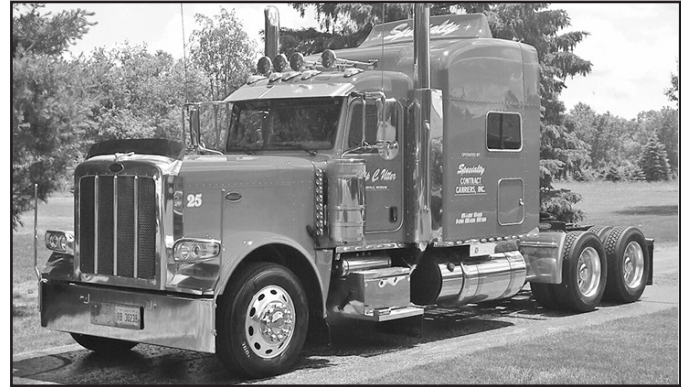
'16 Pete 389 , viper red in color, fully loaded, O/O specs, 78" Unibilt Ultra cab w/platinum int., Cum. ISX 525 hp, 18 spd., 3.55 ratio, air ride, 260" WB, premium steer & drive tires, (10) alum. whls., leather seats & steering whl., keyless entry, Smartnav system, factory aux. heater, recent DPF cleaning, fresh D.O.T., 208,000 miles, this is a very clean 1-owner/1-driver truck in exc. cond. w/all service records, super sharp, like new truck, $139,900.
