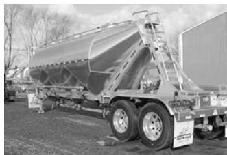
New Tremcar dry bulk trlrs., 1000 cu. ft., air ride, alum. whls.
