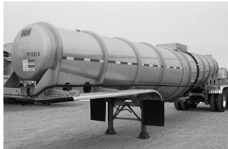
New bulk fertilizer trlrs., 5600-gal., center discharge, air ride susp.
