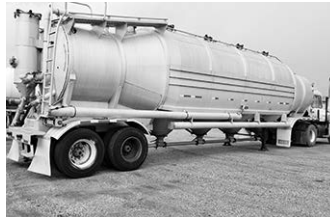
'96 Heil, vacuum, pneumatic, 1625 cu. ft., unit #4354.
