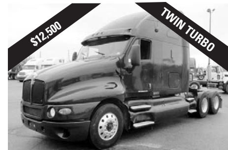
'09 KW T2000 , Cat C15, 435 hp, 13 spd., 12F, 40R, air ride susp., 228" WB, 22.5 tires @ 30-50%, #Y17188.
