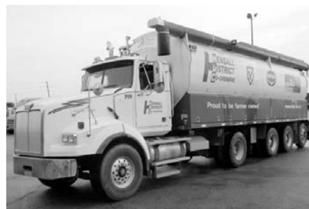
'08 Western Star 4900SA, Agri tank, Mercedes MBE4000, 450 hp, 18 spd. auto., 20F, 46R, air ride susp., 305" WB, 425/65R22.5 frt. tires @ 50%, 11R22.5 rear tires @ 60%, #Y18263.
