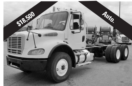
'08 FTL M2-112, Mercedes MBE4000, 350 hp, Allison auto., 18F, 46R, walking beam susp., 248" WB, 315/80R22.5 frt. tires @ 70%, 22.5 rear @ 80%, #Y17202.
