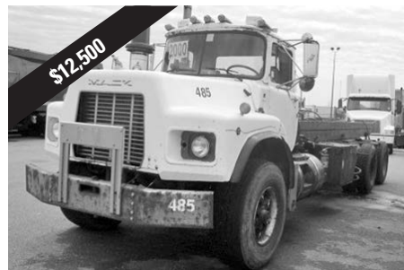
'00 Mack Rolloff, Mack RB688S, Mack E7, 400 hp, 8LL Eaton trans., 20F, 40R, walking beam spg. susp., 218" WB, 425/65R22.5 tires 30% frt., 11R22.5 60% rear, #Y18049.
