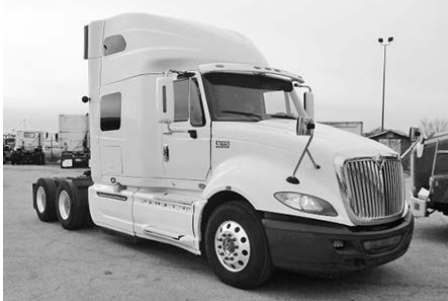
'14 Int'l. ProStar, Cum. ISX, 450 hp, auto., 12F, 40R, air ride susp., 228" WB, 22.5 tires, 70% frt., 30% rear, #Y18106.
