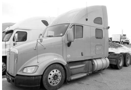
'11 KW T700, Paccar, 430 hp, 12F, 40R, air ride susp., 234" WB, 22.5 tires, frt. @ 70%, rear @ 80%, #Y18100.
