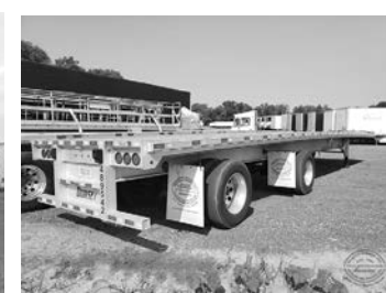
2019 Dorsey 48' aluminum flatbed, 48'x102", aluminum chassis and floor, aluminum 22.5" rims with excellent tires/brakes. Features a fixed spread axle configuration and air ride suspension $34,500.
