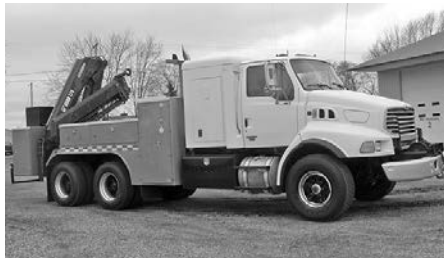
'03 Sterling L9500, C12 Cat, 380 hp, 15 spd. trans., 46R w/lockers, 20F, 175-3 Hiab crane, A/C, 242,000 miles, $38,000.
