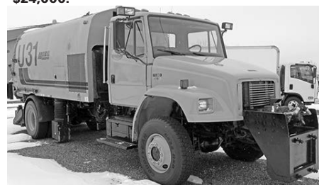
'99 FTL FL80, 8.3L Cum., 250 hp, 4x4, auto., A/C, locking rear axle, dual steer, Athey Mobil sweeper, AV445 16' ft. snow broom, 24,000 miles, $39,000.
