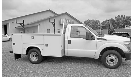
'14 Ford F350, 6.2L V8 gas, auto., A/C, stereo, DRW, RWD, 9' Knapheide utility, 1600# Tommy lift power gate, 38" deep, 48" wide platform, 13,700 GVW, 118,000 miles, $19,995.
