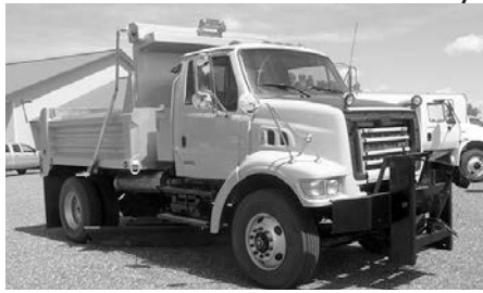
'02 Sterling L7500 Series, 3126 Cat, 275 hp, 5 spd. Allison auto., dbl. PS, air brakes, locking diff., 12' swinging underbelly blade, 10' dump, center pull hoist, 37,700 GVW, 70,000 miles, $39,995.
