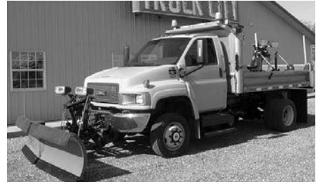
'07 GMC TopKick 5500, 6.6L Duramax dsl., 4x4, auto., A/C, 12' S.S. dump, 10' Western multi position V-plow, broom attachment, 19,500 GVW, 103,000 miles, $49,000.
