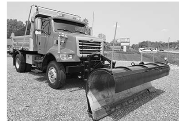
'03 Sterling L8500 , 3126 Cat, 250 hp, 6 spd., Allison auto., A/C, 10' S.S. box, S.S. tailgate, sander, 11' Hydroturn frt. plow, 39,000 GVW, 66,000 miles, $65,000.
