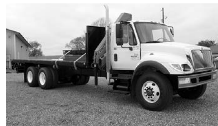
'05 Int'l. 7400, DT466, 300 hp, 8LL trans., dbl. PS, air brakes, tilt, cruise, stereo, air ride seat, 18F, 40R on Hend., 24' bed w/Palfinger 10,000 knuckle boom, 12,000#, 6x4, diff. lock, 26' horizontal reach, 58,000 GVW, 185,000 miles, $28,000.
