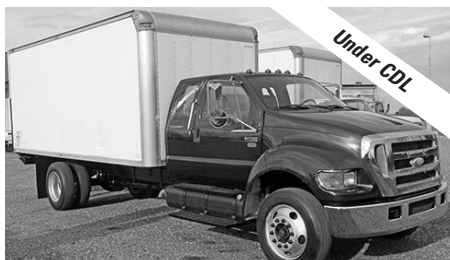
'07 Ford F750, C7 Cat, 275 hp, Allison auto., A/C, cruise, tilt, pwr. windows & locks, air ride seats, 5-pass., 18' van body, 2500 lb. liftgate, 25,999 GVW, 81,000 miles, $32,000.
