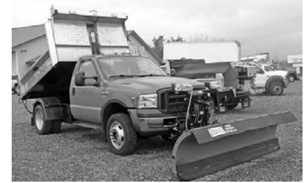
'07 Ford F450, 4WD, V10, auto., 9' Western plow, S.S. dump box w/fold-down sides, tailgate spreader, 38,000 miles, $45,000.
