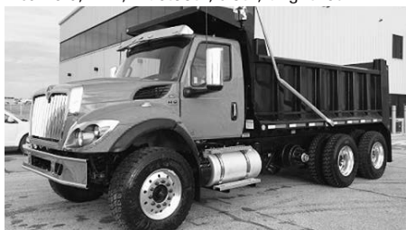
HV607 tri-axle , L9-370, 8LL trans., 16F, 40R, quad lock, 15' Galion dump, elec. tarp, pintle.
