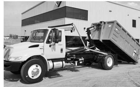
'13 Int'l. 4300 w/new SL-180 Swaploader , pintle hitch, elec. tarp, under CDL, 116,000 miles, nice unit.
