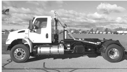
New '19 Int'l. MV607 , 280 hp Cum., auto., air ride, 33,000 GVW, Swaploader SL185 hook lift w/ Roll-Rite elec. tarp, ready to work.
