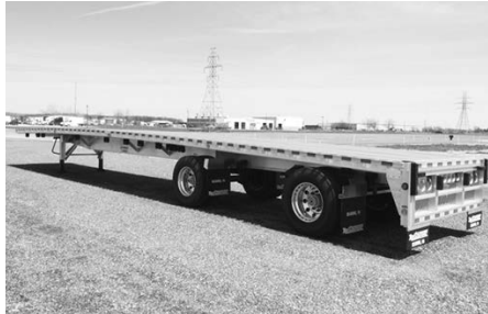
Reitnauer 53' Big Bubba , (12) slgd. winches, 11R22.5 Michelins, slgd. rear axle, (3) wood nailers, California & BC legal.
