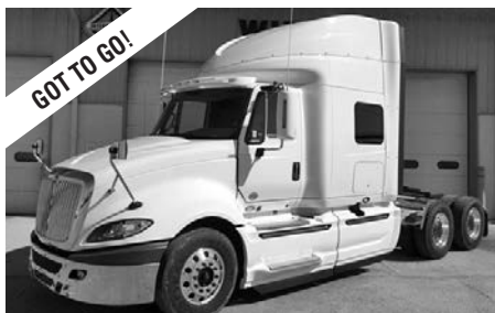
'17 ProStar Eagle , ISX 450 hp, 13 spd., 230" WB, 3.36 ratio, 73" hi-rise, dual 120-gal., nice specs.
