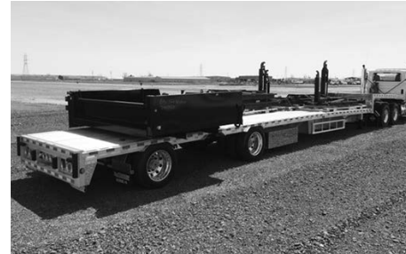
Reitnauer 53' drop deck , (16) slgd. winches, dunnage box, (2) tool boxes, 255/70R22.5 Michelins, slgd. rear axle.
