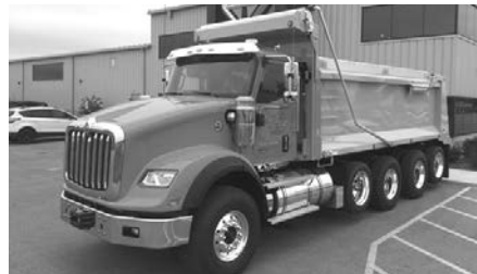
HX620 quad chassis , Cum. X15, 565 hp, 18 spd., 20F, 46R, 207" WB, 1/2" frame rail, chassis or tri/quad dump - complete build handled in-house!
