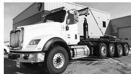
New HX620 , X15-485 hp, Allison 4500RDS, 20F, 46R, Hend., full lockers, SL-520 Swaploader, adj. pivot tarp, (2) steerable lifts, hitch.
