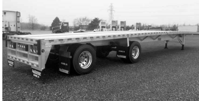
53'x102" Big Bubba , sldg. rear axle, (12) sldg. winches, (3) wood nailers, pol. alum. whls., CA & BC legal.
