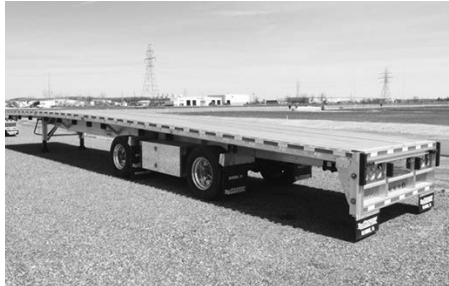
Reitnauer 53' Big Bubba , (12) slgd. winches, 445/50R22.5 Michelins, Tire Max Pro inflation, (2) tool boxes, rear dunnage w/door, CA legal.
