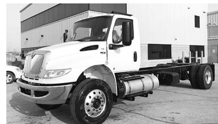
MV607 chassis , fresh new design inside & out, 26,000 & 33,000 GVW, Cum. B 6.7, Allison, air brakes, air ride, we can alter/upfit to your needs.
