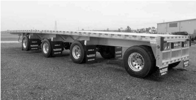
48'x102" Bigger Bubba , quad axle, (2) lifts, full coil pkg., (4) wood nailers, pol. alum., Michelin XZE2.
