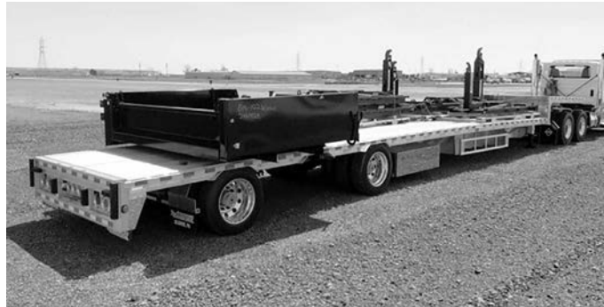
53'x102" DropMiser , sldg. axle, (16) sldg. winches, dunnage box, (2) tool boxes, 255/70R22.5 Michelin, pol. alum. whls.
