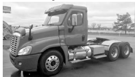
'11 FTL Cascadia , ISX-450, Jake, 10 spd. manual, 12F, 40R, air ride, dual 100-gal. fuel tanks, (10) alum. whls., 481,000 miles, nice tractor.
