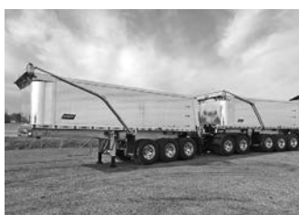
Stargate alum. triple 10 , alum. frame, 96" wide, 60" sides, liners, Roll-Rite elec. tarps, push bumper.
