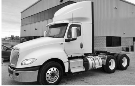
'18 Int'l. LT625 , X15-450 Efficiency, Jake, 10 spd., 3.36 ratio, 177" WB, roof fairing, dual 80-gal. fuel tanks, alum. frt., LP22.5.
