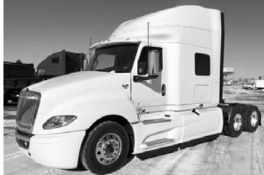
'19 LT slpr. , Cum. X15-450 Smart Advantage, Endurant 12 spd. automated, 2.79 ratio, Pred. cruise, Espar bunk heater.
