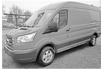
'17 Transit MR , mid-roof, 3.7L gas, glass side & rear door, red in color.
