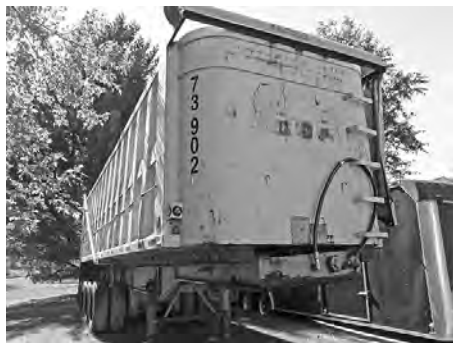
'87 Dorsey high side dump, as you can see, the right side is bent from when the door opened & it rolled, cyl. pin came out of btm., that's why it rolled over, cyl. needs to be repacked, not bent, plenty of room for a 5th axle to go under, all (16) tires match & about 85% rubber, minor tarp damage, asking $5,500 or make an offer. (313) 215-4291
