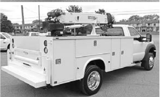
'13 Ford F450, 12' Utility service body, Stellar EC3200 crane, 15' horizontal reach, crane rating 11,500 ft.-lb., remote controls, 6.8L V10, A/C, auto., new tires, 70% brakes, bed Rhino lined, no rust, Alabama truck, serviced & ready to go, about as nice as they come, it's a 9.5, 95,300 miles, financing available, $42,900. Doug (248) 867-4049 7 Days
