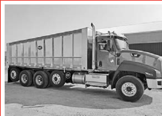
New '16 CT660L, CT13 eng., 475 hp, Cat CX31 auto., 20F, 46R, (2) steerable lift axles, color gray metallic, MAC 22' alum. body, Roll Rite tarp system, liner, pup hitch.
